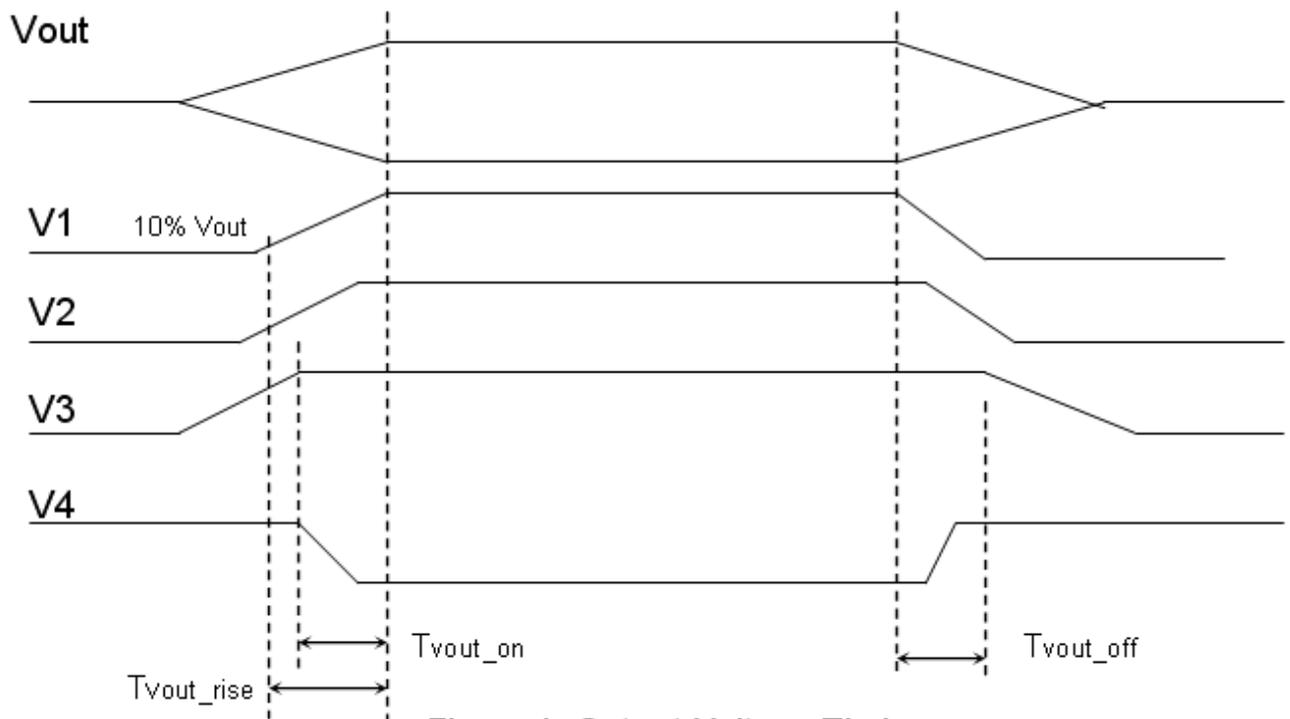
Figure 1: Output Voltage Timing
